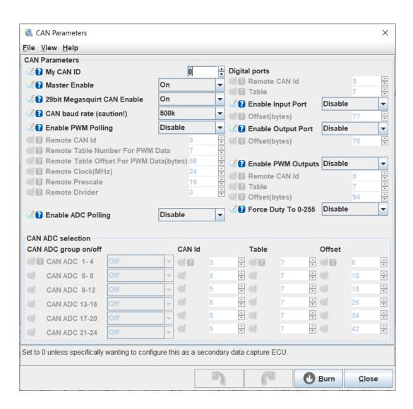
Next, under CAN-Bus/Test Modes menu, select "CAN Receiving" menu and configure as seen in the figure below. CAN ADC01 is the Pitch channel; CAN ADC02 is Pitch Velocity; CAN ADC03 is X-Accel and CAN ADC04 is Corrected X-Accel; CAN ADC05 is the IMU Temperature. Note that you may have devices that already use CANADC01
